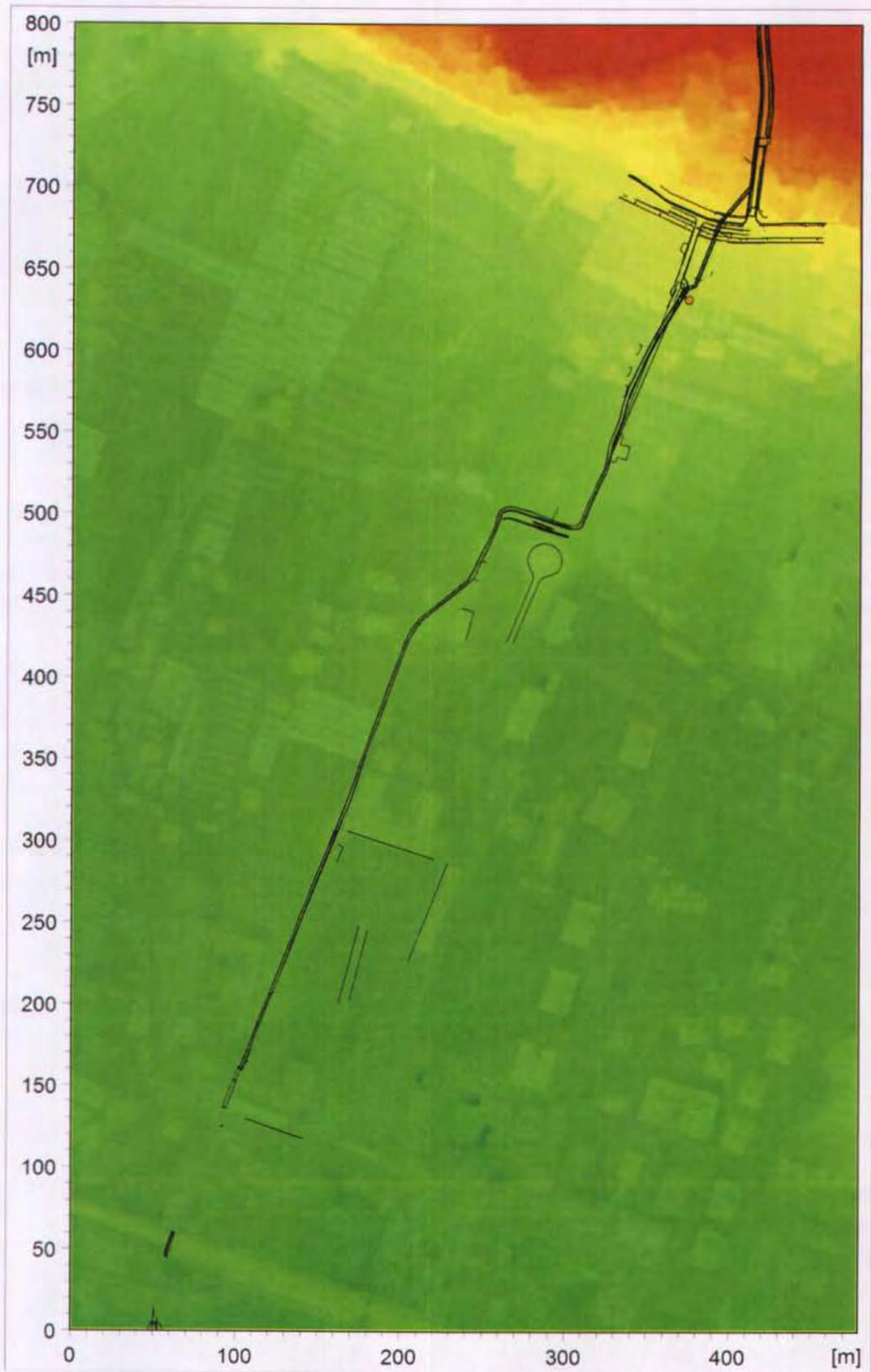
Figura 34 - Batimetria del modello 2D a maglia 1,0x1,0 m.
